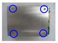
Step 2: Fasten the 4 pieces of anti- vibration Rubbers on the HDD bracket.
